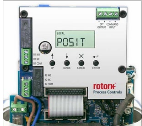
PCB & Terminal Board (Inside CMR Enclosure)
